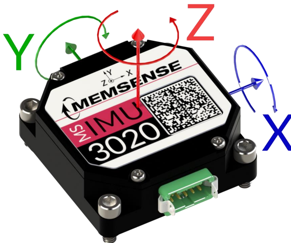
Figure 2 – MS-IMU3020 coordinate system
